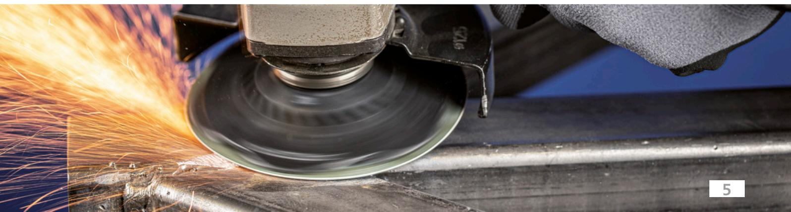
The extensive range of fibre discs provides the optimum product for any machining application, from coarse to fine grinding. PFERD provides fibre discs with various grit sizes, abrasives and dimensions. In accordance with ISO 16057, PFERD fibre discs are manufactured in shape A2, type F, and designated "vulcanized fibre discs".
