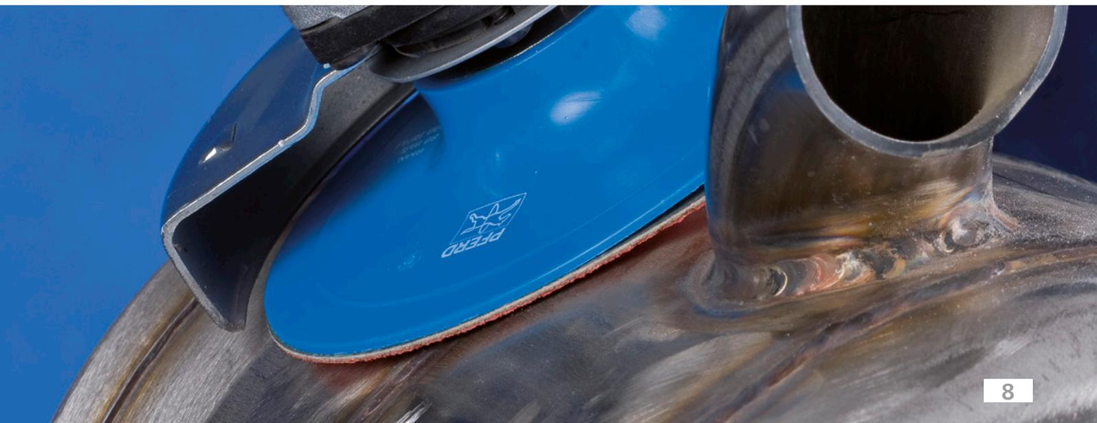
The COMBIDISC® product range contains a wide selection of grinding products for surface finishing. From coarse machining and surface texturing to face-down mirror polishing – the range provides the best product, even for complicated applications.
